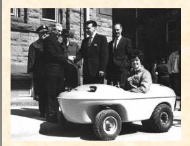
A Penguin is a 4 wheeled, two seated amphibious vehicle. Penguins were designed to be used by sportsmen, industry and the armed forces. Trailers and front wheel clip on skis were available options. Top speeds of up to 40 mph were claimed on land, and 4 mph on water!
